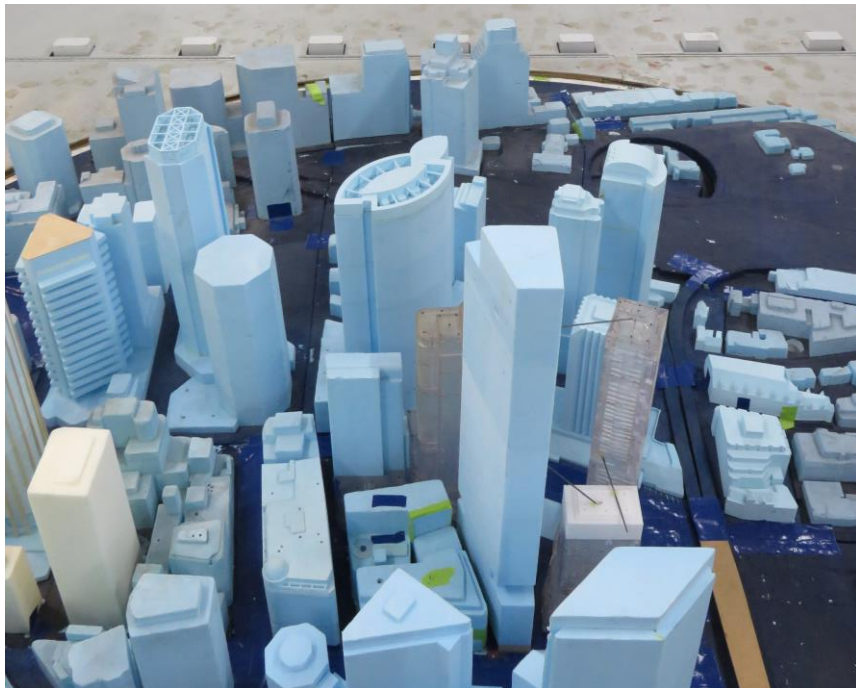
Figure 15: Close-up of Configuration A model in the wind tunnel viewed from the east
